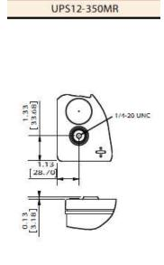
\*All dimensions in inches (mm). All dimensions are for reference only. Contact a C&D Representative for complete dimension information. NOTE: Batteries to be mounted with 0.5 in (1.25 cm) spacing minimum and free air ventilation. UPS
